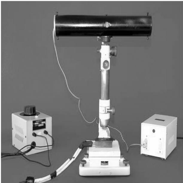
FIGURE 8 Autocollimator for the determination of variation of the angle of the small angle cell with temperature.
